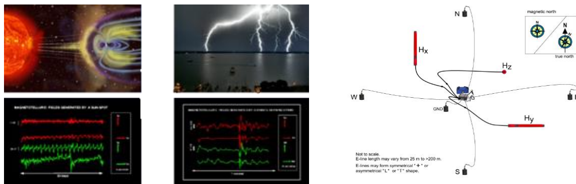
Figure 1 - Sources of EM energy for MTS and MVP methods and a scheme for field recording of a natural alternative electromagnetic (NAEM) field
